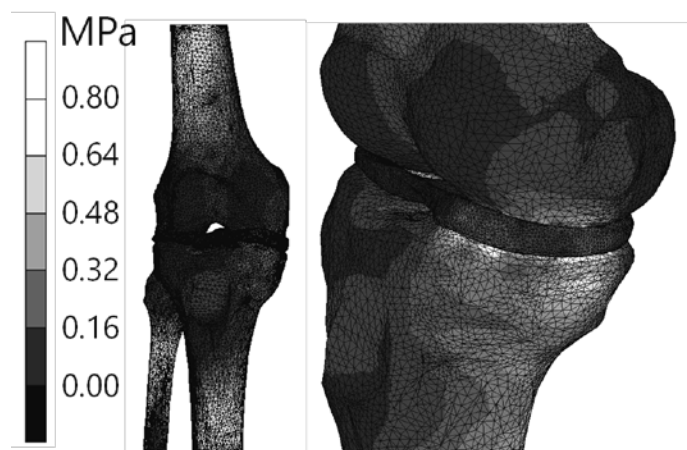
Fig. 7 Distribution of equivalent of Mises stress
