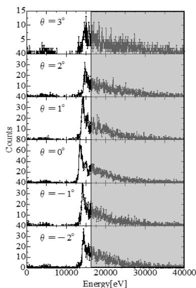
Figure 1. Kinetic energy distributions of transmitted Ar<sup>6+</sup> ions after injection into the CGC.
