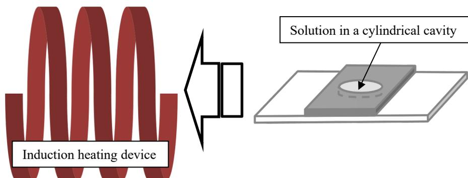
Figure 1. Outline of the experimental setup. Solution of C<sub>60</sub> molecules/sulphur or C<sub>60</sub>/sulphur/magnetic nanoparticles dispersed in benzene is introduced in a cylindrical cavity, which is placed on a glass substrate. The bottom of the test cell is heated or the test cell is subjected to an ac magnetic field.
