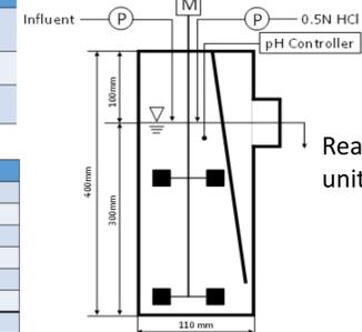
Fig.3 Schematic Reactor
